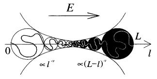
Fig. 2. Equilibrium conformation of a symmetric diblock polyampholyte (SDP) in an external electrical field (tug of war). The chain consists of a string of Pincus blobs of different sizes  $\xi_{n(l)}$  and the global shape is trumpet-like at both ends forces (blob sizes) decrease (increase) from the grafted site to the free end, so that the chain attains a trumpet-like shape. Thus a polymer exposed to a tug of the war shows a similar shape, having, however, two trumpet-like ends.
