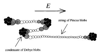
Fig. 6. Configuration of a randomly charged PA for large field strength  $E > E_c$ . Schematically depicted is a typical conformation above the instability range. The chain consists of strongly stretched portions (strings of Pincus blobs) and of condensates of Debye blobs; the latter are to be found at the ends and at turning points of the zig-zag conformation (see text for details)
