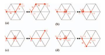
FIG. 1. Schematic depiction of the Monte Carlo moves. The arrows denote the bond vectors, where an arrow that ends and starts at the same monomer is an element of stored length. (a) and (b) Instances of corner moves. (c) The end moves. (d) An example of a transversal move.
