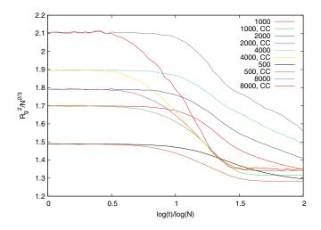
FIG. 12. Final radius of gyration  $R_g$  after swelling the globules that have been relaxed for t time steps, either with or without chain crossing moves. Each polymer globule is swelled for 2N time steps, before its radius of gyration is measured. The ones with chain crossing are indicated in the plot by CC in the key. Globules with few entanglements will swell much more easily than ones with many of them.
