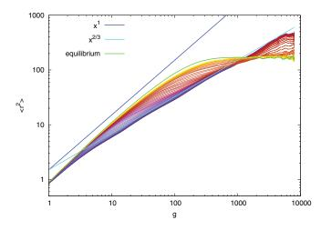
FIG. 9. Equilibration without chain crossing of a N = 8000 smooth random FCC fractal. Chain crossing is not allowed in this simulation. This is a mean square displacement versus the genomic distance g = |i - j| plot. The time starts with the black curve at t = 1 and increases exponentially in 50 steps to  $t = N^2$ .
