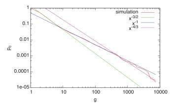
FIG. 15. Contact probability  $p_c$  as a function of genomic distance g at  $t = N^{0.92}$ , for a polymer of length N = 8000. The lines indicate the perceived "zigzag" as elaborated in the main text. The full time development is shown in Fig. 7.
