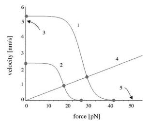
**Figure 7.7** Force–velocity relations. Curves 1 and 2 show the relation between transcription-velocity and externally applied load of RNA polymerase in two different cases. Lines 3 to 5 give the force–velocity relation for nucleosomes under an externally imposed force, again for three different cases.
